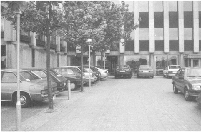
Fig. 7. A dense urban parking area uses diverse paving types, some of which allow water to filter into the ground.
